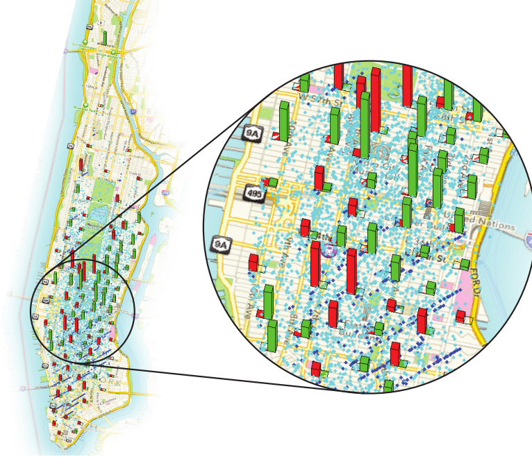
Fig. 4. Simulation environment with 100 stations in Manhattan. Red bars indicate waiting customers, green bars indicate available vehicles, cyan dots are vehicles traveling with passengers and blue dots are rebalancing vehicles.
