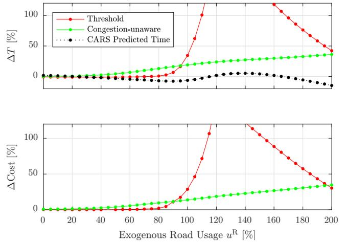
Fig. 5. Relative deviation of the two baseline solutions compared to CARS. The upper plot also shows the relative error of the CARS predicted time.
