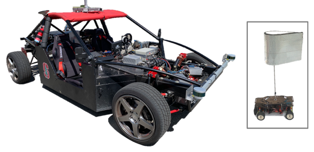
Figure 8. X1: a steer-by-wire experimental vehicle platform. The 1/10-scale RC car has a mast that is visible to the LiDARs.
