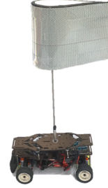
Fig. 5: 1/10-scale RC car with LiDAR-visible mast.
