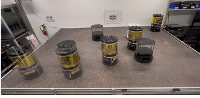
Fig. 3: Free flyer testbed and real-world execution of the FT-TTO trajectory in Fig. 2c. Transparency identifies the time progression from the start (faded) to the end (opaque) of the trajectory.
