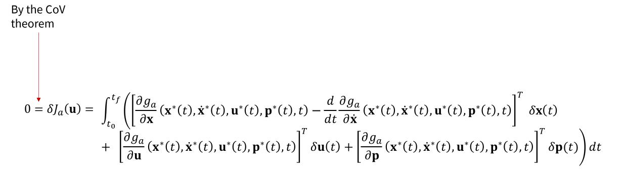
On an extremal, by applying the fundamental theorem of the CoV
