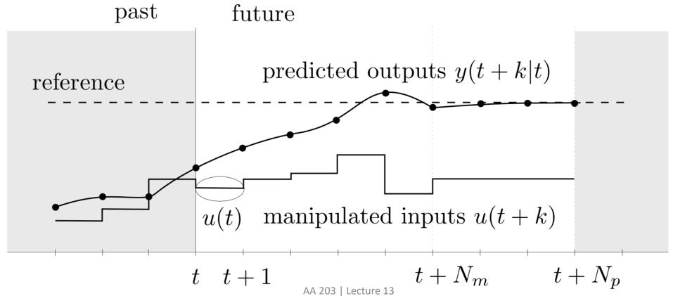
Model predictive control (or, more broadly, receding horizon control) entails solving finite-time optimal control problems in a receding horizon fashion
