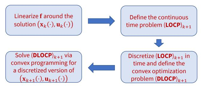
$$(\text{DLOCP})_{k+1} \qquad \min_{(\mathbf{x}_{i},\mathbf{u}_{i})} \sum_{i=0}^{N-1} h_{i}g(\mathbf{x}_{i},\mathbf{u}_{i},t_{i}) \\ \mathbf{x}_{i+1} = \mathbf{x}_{i} + h_{i}\mathbf{f}_{k+1}(\mathbf{x}_{i},\mathbf{u}_{i},t_{i}), i = 0, \dots, N-1 \\ \mathbf{u}_{i} \in U, i = 0, \dots, N-1, \qquad \mathbf{x}_{N} = \mathbf{x}_{f}$$
