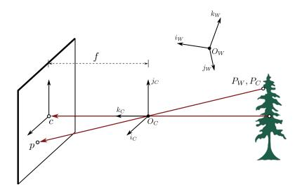
Figure 8.1: Graphical representation of the pinhole camera model. In this model the point  $O_C$  is the camera center, c is the image center, and f is the focal length of the camera. It is assumed that all light rays from point P in the scene pass through point  $O_C$  and are captured on the image plane at point p.
