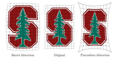
Figure 8.4: Different kinds of radial distortions that are seen in real lenses, which may affect the accuracy of the pinhole camera model.
