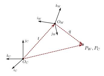
Figure 8.3: A depiction of the point P expressed either in camera coordinates,  $P_C$ , or in world frame coordinates,  $P_W$ . The world frame origin is denoted by  $O_W$  and the camera frame origin is denoted by  $O_C$ .
