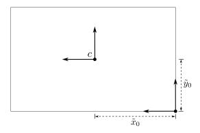
Figure 8.2: A new reference frame with coordinates denoted by  $(\cdot)$  is defined with its origin in the lower corner of the image plane. The image center coordinates in this new frame are denoted  $(\tilde{x}_0, \tilde{y}_0)$ .
