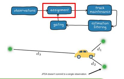
*Example*: JPDA tracker calculates the possibility of association between track  $T_1$  and observations  $O_1$ ,  $O_2$  and  $O_3$
