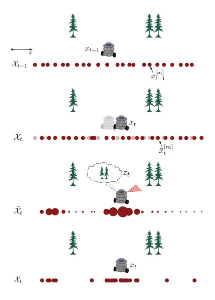
Figure 15.1: Particle filter used for robot localization. The initial set of particles are first updated according to the transition model, and then weighted according to the observation. Finally, a new set of particles is generated through weighted resampling.
