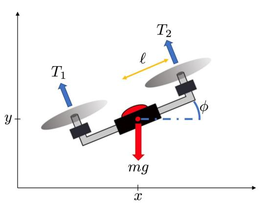
$$\min \int_0^{t_f} T_1(t)^2 + T_2(t)^2 dt$$
