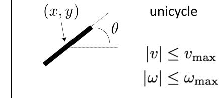
$$\begin{pmatrix} \dot{x} \\ \dot{y} \\ \dot{\theta} \end{pmatrix} = \begin{pmatrix} \frac{r}{2}(\omega_l + \omega_r)\cos\theta \\ \frac{r}{2}(\omega_l + \omega_r)\sin\theta \\ \frac{r}{L}(\omega_r - \omega_l) \end{pmatrix}$$
