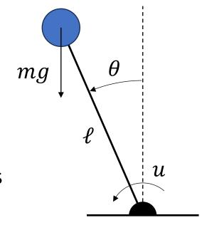
• This is close to a double-integrator! We could try  $\frac{1}{m\ell^2}u = -\left(\frac{g}{\ell} + \kappa_p\right)\theta - \kappa_d\dot{\theta}$  to stabilize the pendulum near the upright equilibrium
